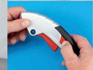
Engage the safety lock when not using the knife ■.
