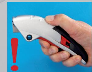
...and rotate the squeeze lever back into the handle until it snaps in place. Unlock knife ■ and test the squeeze lever to be sure it is working properly.
